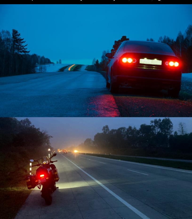
View of car and motorcycle from behind during rain. Note the car has two separated lights, plus a reflective license plate. The motorcycles have only one, smaller, light view.
