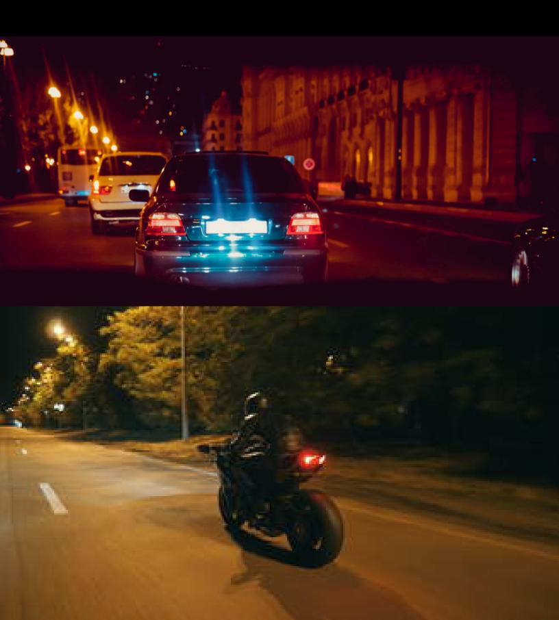
View of car and motorcycle from behind at night on the side of the road. Note the car has two separated lights, plus a reflective license plate. The motorcycle has only one, smaller, light view.
